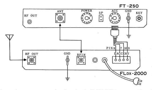
Diagram shows correct connections for using the FL-DX-2000 Linear Amplifier with the FT-250.
