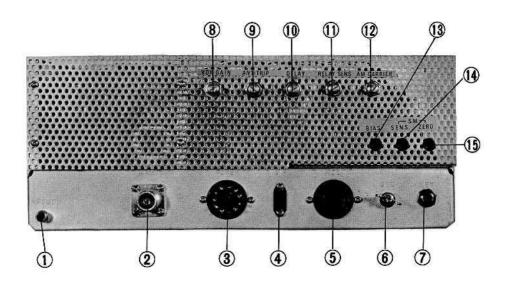
1. RF Out Provides low level RF drive for FTV-650 VHF transverter.
